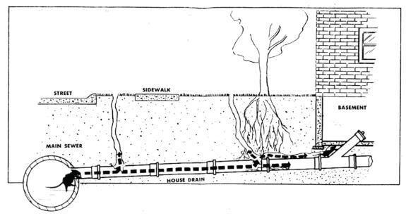
Figure 1: Rats leave the main sewer and access a home through a lateral line.
